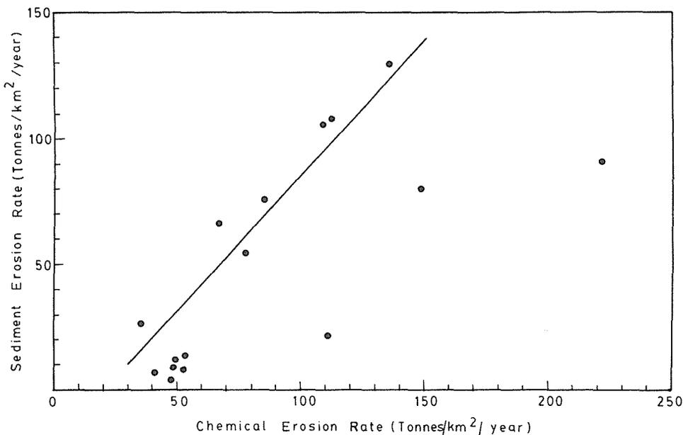
Fig 3 Sediment erosion/chemical erosion relationship for the Krishna river basin.
