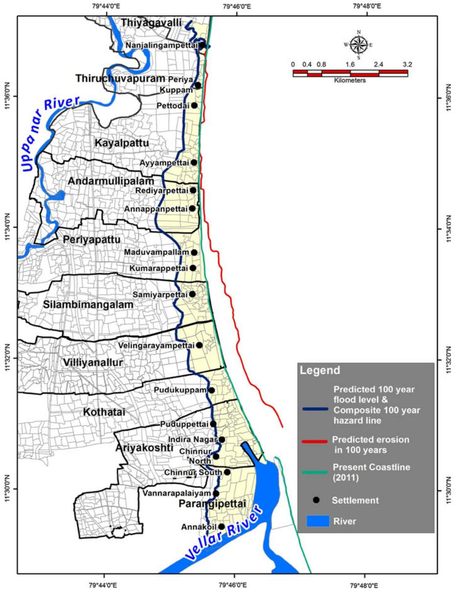
**Fig. 6** Lines depicting the predicted erosion in 100 years, predicted 100-year flood level and the Composite 100-year hazard line on a cadastral map of the Cuddalore coast
