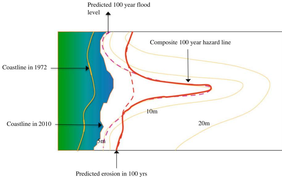
**Fig. 2** Concept of composite hazard line (after Pethick 2009)
