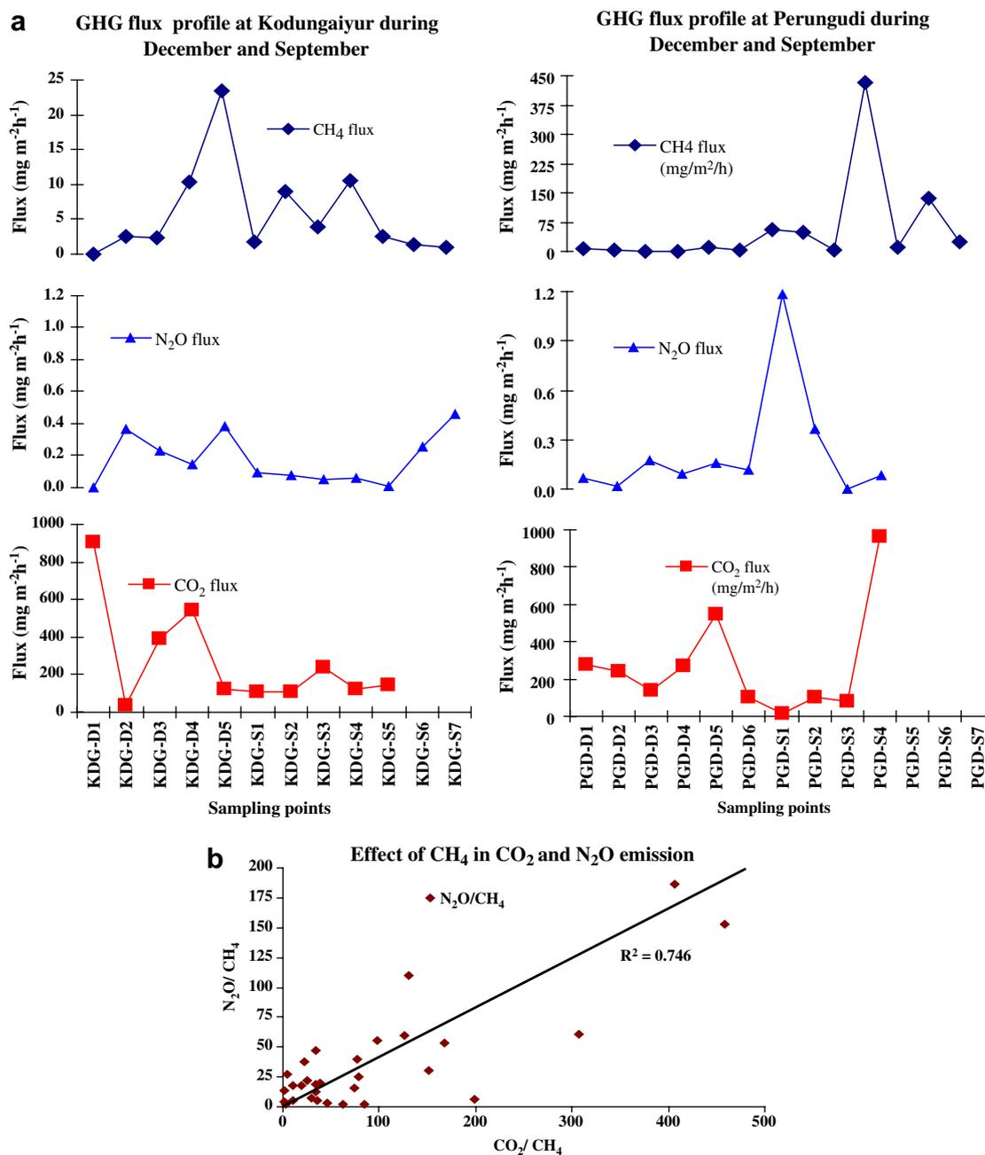
Fig. 2. Emission fluxes of gas and their interrelationship (a) Emission fluxes in landfills (PGD = Perungudi, KDG = Kodungaiyur, D = December, S = September); (b) effect of CH<sub>4</sub> on CO<sub>2</sub> and N<sub>2</sub>O emissions.
